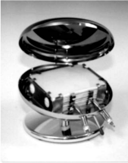
Fig. 8.42 Photograph of Ni-H 2 cell components prior to final assembly.
