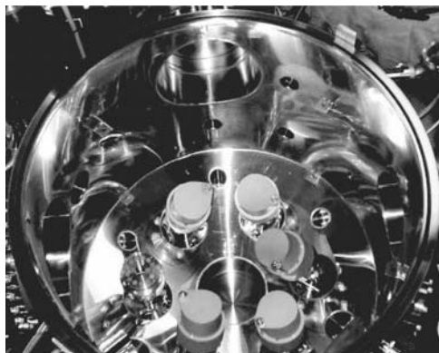
Fig. 7.37 Photograph of the sputtering chamber showing six magnetron sources. Five of them are covered with a shutter, one is uncovered (on the left) showing the magnets within the source. The sources are at various tilt angles.
