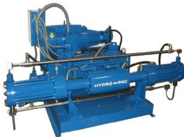
Figure 8: Hydro-Pac Two Stage Hydrogen Compressor
