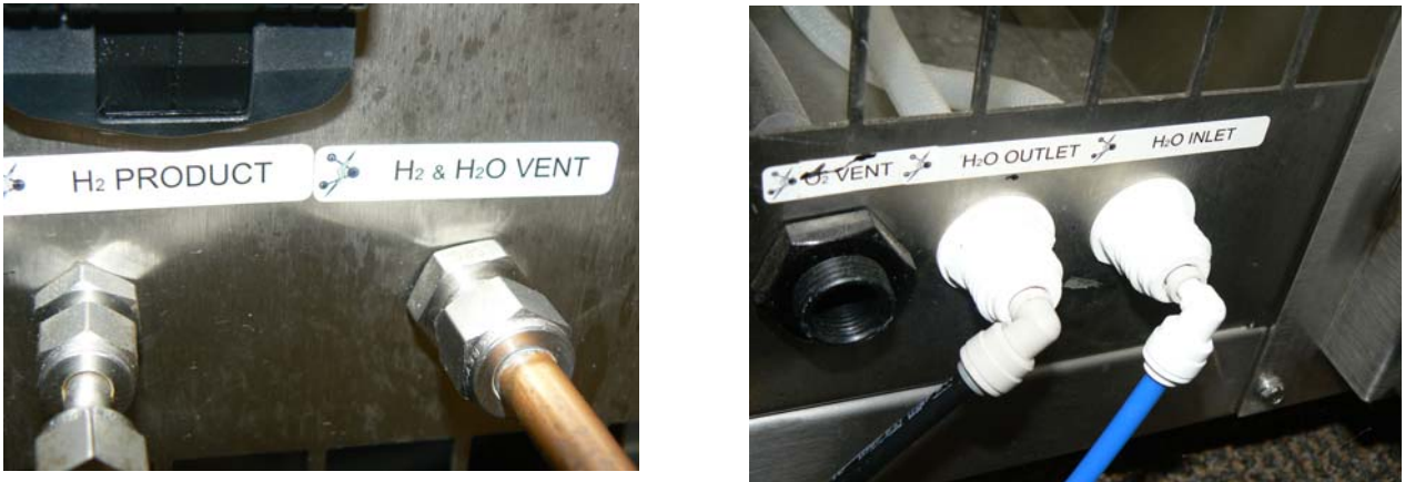
Figure 12: Terminal Connections for Relion Fuel Cell and I comms Interface screen
