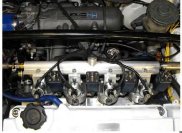
Our whole operating system is not so different from the conventional engine. The part we modify is the cylinder head and the infrastructure to get the hydrogen from tank to engine.
