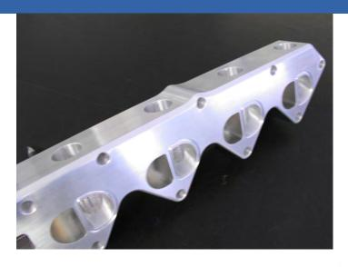
This flange optimizes the separation between air and hydrogen before entering the combustion chamber.
