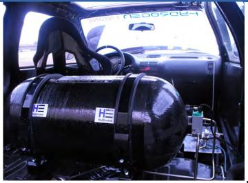
Our hydrogen is currently stored inside a cylinder tank (type V074H350X8) made by Dynetek, Germany.
