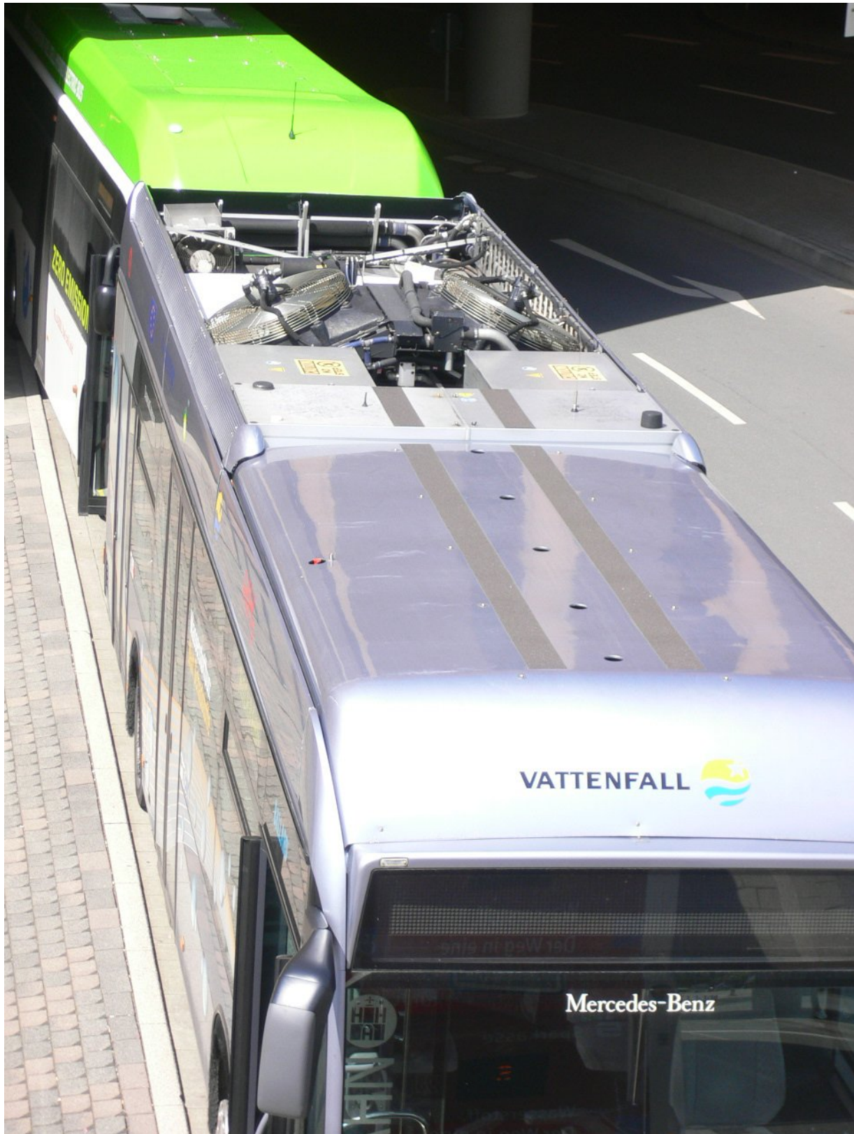
Topside detail of the Daimler – note they have stayed with the hydraulic fans. VanHool bus in green behind.
