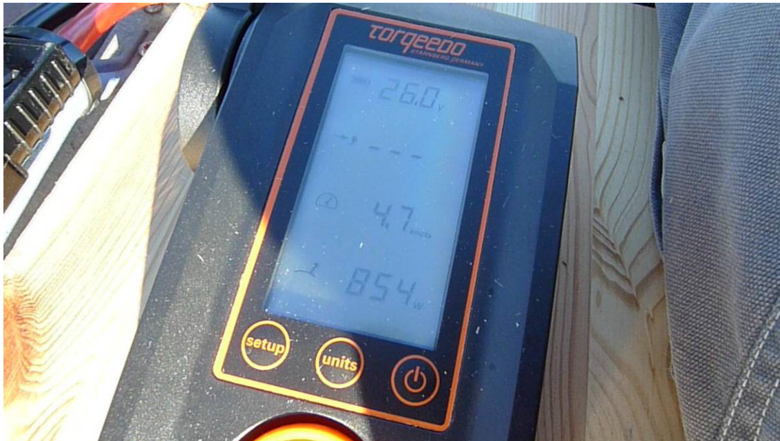
Throttle. Voltage: 26,0 V. Speed: 4,7 knots. Power: 854 W.
