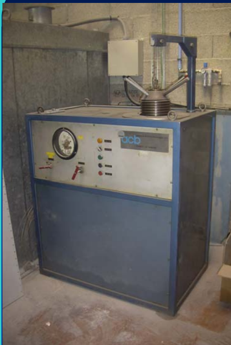
Isostatic cold pressing up to 4000 bars
